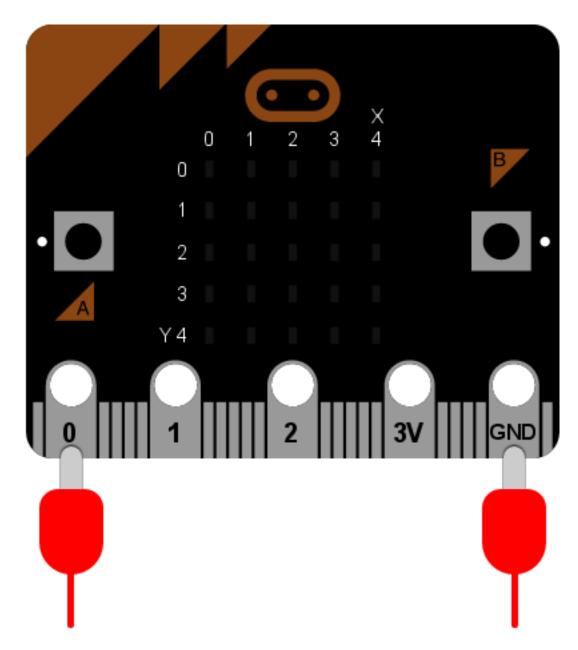
The wire from pin 0 should be attached to the positive connector on the buzzer and the wire from GND to the negative connector.
